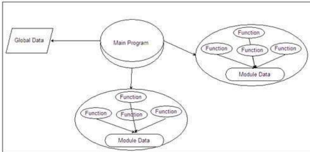
Modularizing a design helps to plan the development in a more effective manner, accommodate changes easily, conduct testing and debugging effectively and efficiently, and conduct maintenance work without adversely affecting the functioning of the software.
