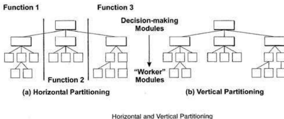
In **vertical partitioning**, the functionality is distributed among the modules--in a top-down manner. The modules at the top level called **control modules** perform the decision-making and do little processing whereas the modules at the low level called **worker modules** perform all input, computation and output tasks.
