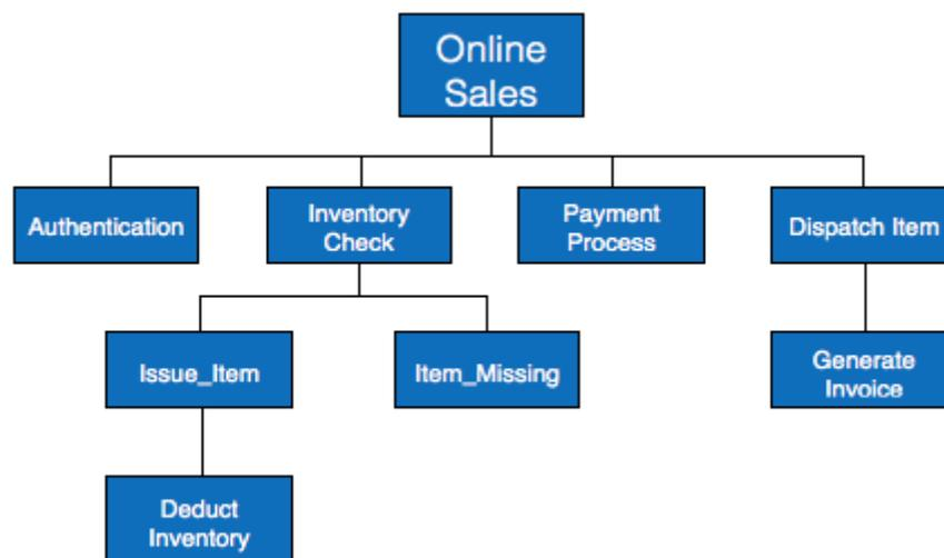
In contrast to IPO (Input Process Output) diagram, which depicts the flow of control and data in a module, HIPO does not provide any information about data flow or control flow.
